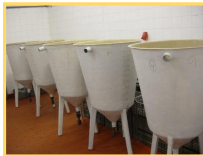
Figure 5 – Batch system. Cylinder-conical tanks for larval rearing.
