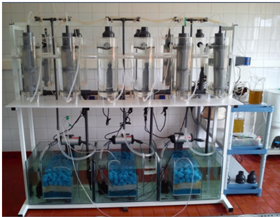
Figure 6 Recirculating aquaculture system (RAS) for larval rearing.
