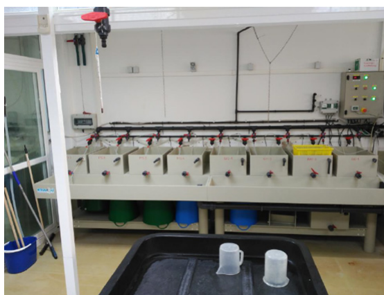
Figure 29. Setting of the 8 conditioning trays, with the 4 FTS trays (left) and the 4 RAS trays (right). The upper red taps correspond to the RAS circuit and the lower ones to the FTS.
