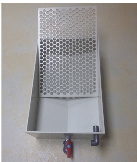
Figure 28 Conditioning tray with perforated base and sloping bottom
