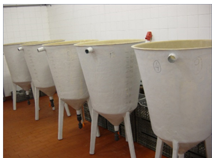
Figure 5 Batch system. Cylinder-conical tanks for larval rearing
