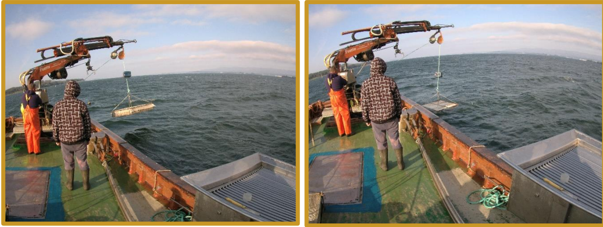
Figure 4. A frame structure with six boxes in the process of submersion in Lombos do Ulla.
