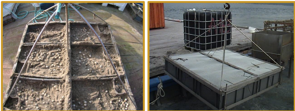
Figure 3. Left: six plastic boxes filled with shellfish-bed sediment, arranged within a frame structure on board a ship. The marked cockles visible on the sediment had just been set and they would burrow within the sediment once boxes were submerged. Compartments delimited with a
