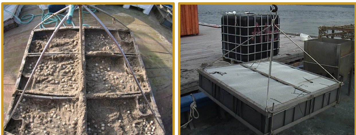
Figure 3. Left: six plastic boxes filled with shellfish-bed sediment, arranged within a frame structure on board a ship. The marked cockles visible on the sediment had just been set and they would burrow within the sediment once boxes were submerged. Compartments delimited with a net, envisaged for mortality estimation, are visible in one corner of each box. Right: the six boxes covered with a net to avoid predation.
