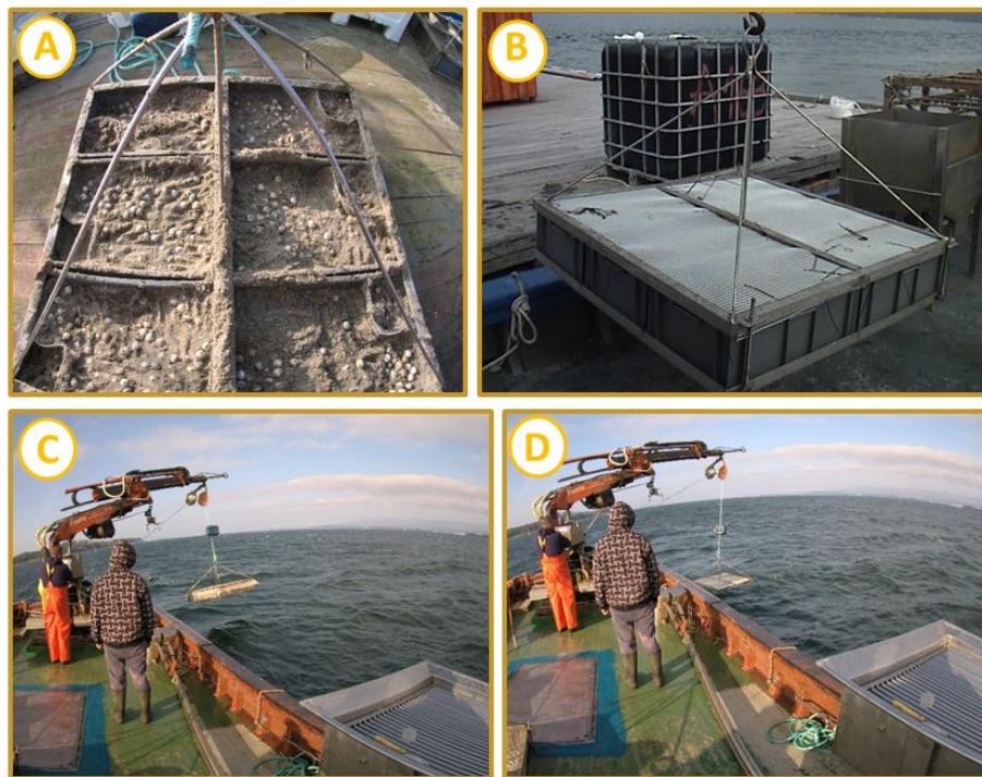
Fig. 2. A: six plastic boxes filled with shellfish-bed sediment, arranged within a frame structure; the cockles on the sediment had just been set and they would burrow within the sediment once boxes were submerged. B: the six boxes covered with a net to avoid predation. C and D: a frame structure with six boxes in the process of submersion in Lombos do Ulla.
